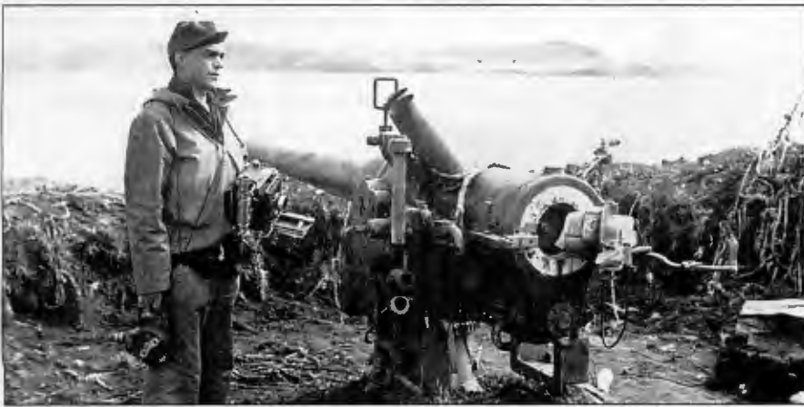
With more than a year to dig in, the Japanese left behind well-prepared coastal batteries, entrenched artillery such as this Type 41 75mm mountain gun, and extensive AA artillery and automatic guns. Only troops and small arms were evacuated.
